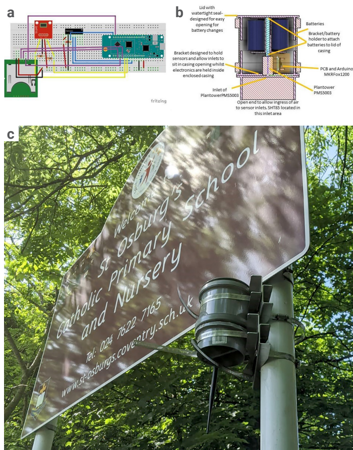
Figure 9: a) Fritzing diagram of the breadboard-based prototype for the AltasensePM. b) A diagram of the custom casing. c) An AltasensePM device deployed outside a school
